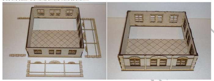
Turn  $2^{nd}$  floor piece upside down and glue three pegs in place. This will keep the  $2^{nd}$  floor piece in place and allow lifting it up to reach the interior.
