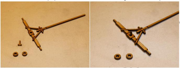
Glue big ring onto matching ring of undercarriage. Complete base of cart by gluing axle in place, then add undercarriage as shown.
