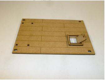
Glue the two frame pieces without holes in place as shown. Insert the door pins in the frame holes and glue into the roof opening from the top! Then finish by adding the surrounding frame piece.
