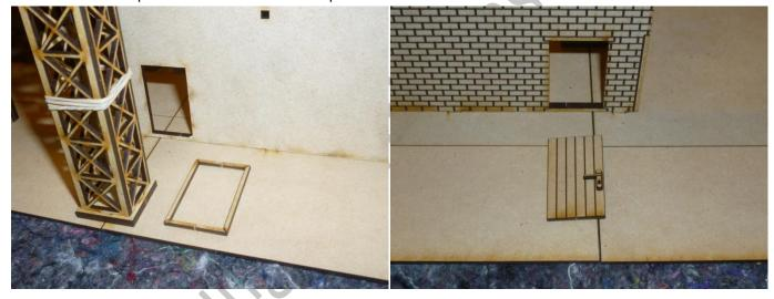
Glue two sliding door rail supports in place as shown.
