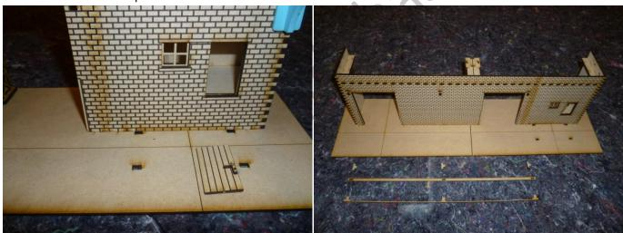
Glue three sliding door rail supports in place as shown.
