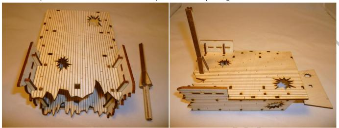
Glue together the two main parts of the rudder. Glue the three supports into the slots as shown.
