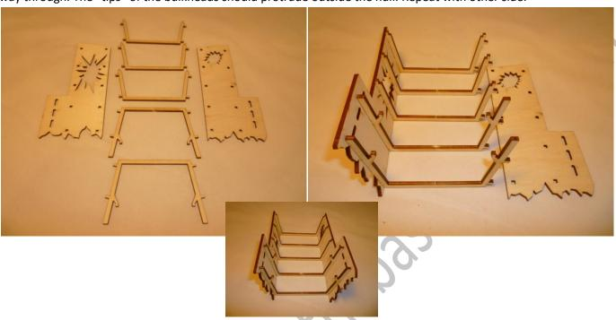
Glue the lower deck into the hull. Then glue upper deck into the hull.
