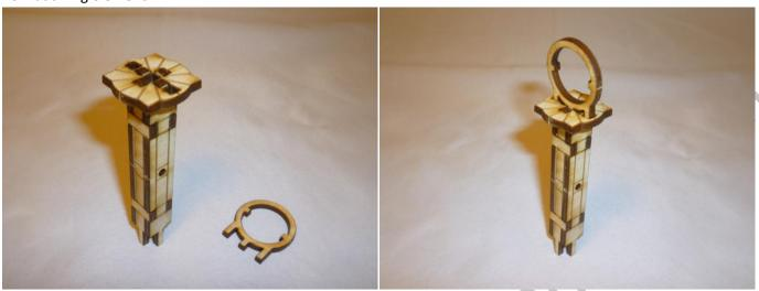
Glue two faces back to back. Insert piece centered into ring element.
